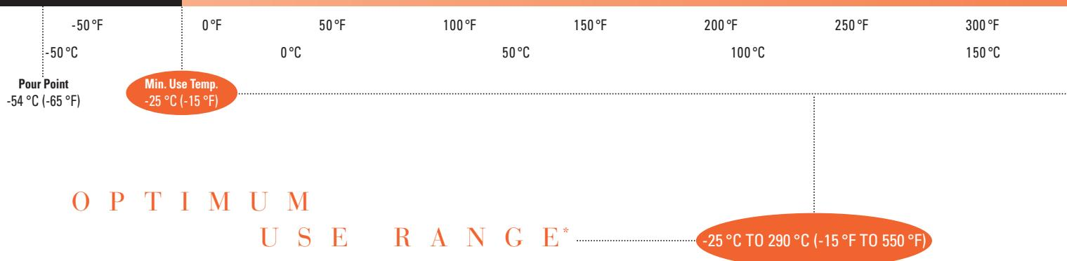
Therminol® 55 is a unique, synthetic heat transfer fluid designed to provide reliable, consistent heat transfer performance over a long life.
